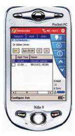
The WinScribe PDA application communicates with the WinScribe server via HTTP or HTTPS. This allows authors to dictate while on the move and have the voice files automatically sent to the server whenever a connection is present. Connection methods that allow us to work this way include Wireless technology, GSM/ GPRS/Bluetooth/ Cellular, etc.
